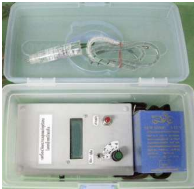
Figure1 Electrical capacitance meter of monthong durian
